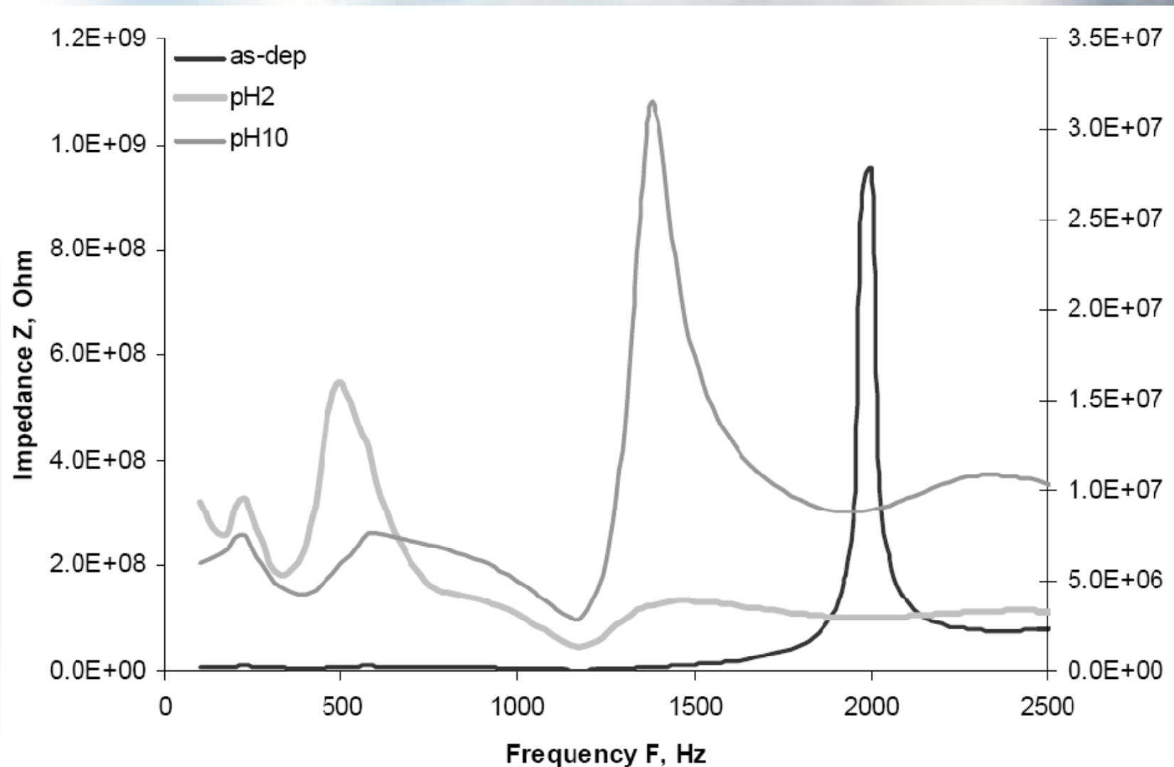
**Change in the resonant frequency and impedance values of 25 wt.%  $\text{Bi}_2\text{O}_3$  and 75 wt.%  $\text{Nb}_2\text{O}_5$  mixed sensor as a result of pH 2 and pH 10.**
