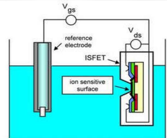
Schematic representation of an ISFET pH measuring system
