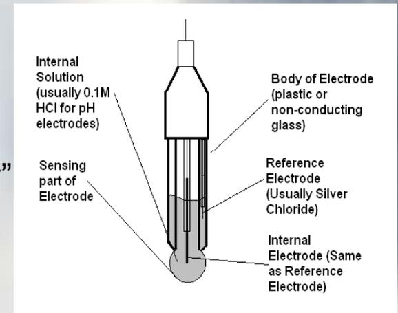
*Schematic Diagram of Simple Glass Electrode*
