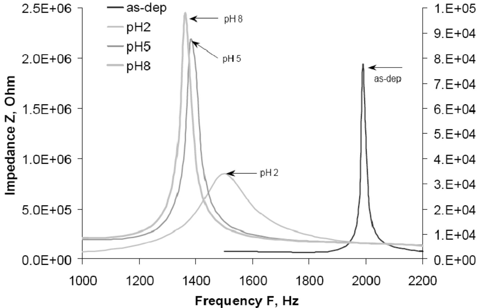
**Change in the resonant frequency and impedance values of the  $\text{Bi}_2\text{O}_3$  thick film pH sensor.**
