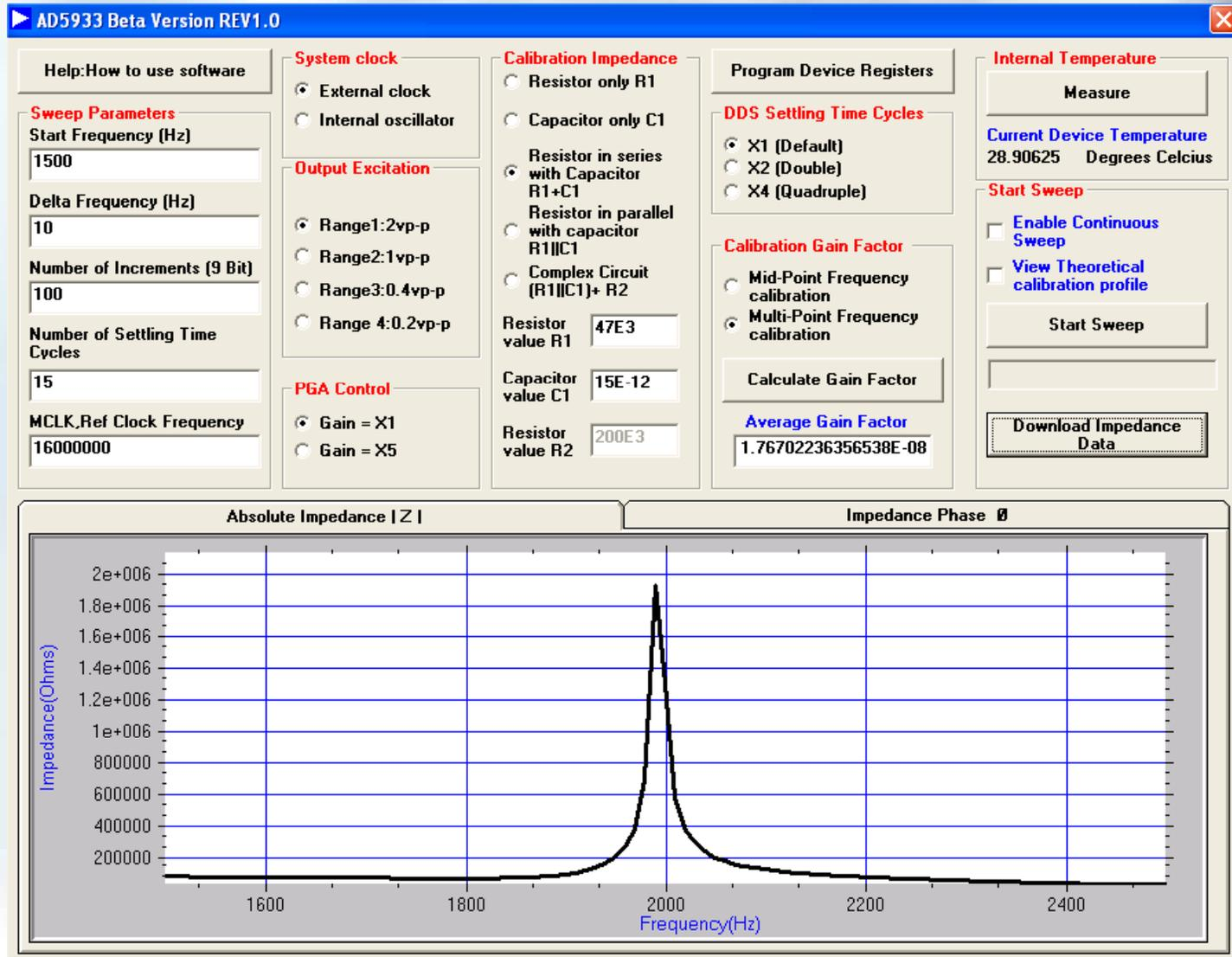
**Graphical representation of AD5933 impedance converter software interface**
