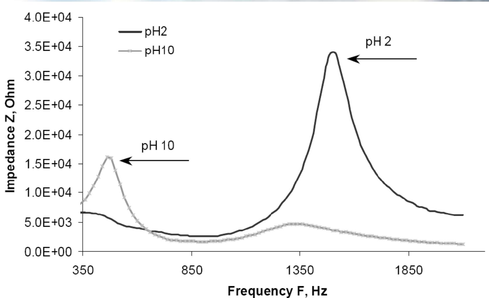
**Change in the resonant frequency and impedance values of the  $\text{Bi}_2\text{O}_3$  thick film sensor as a result of pH 2 and pH 10.**
