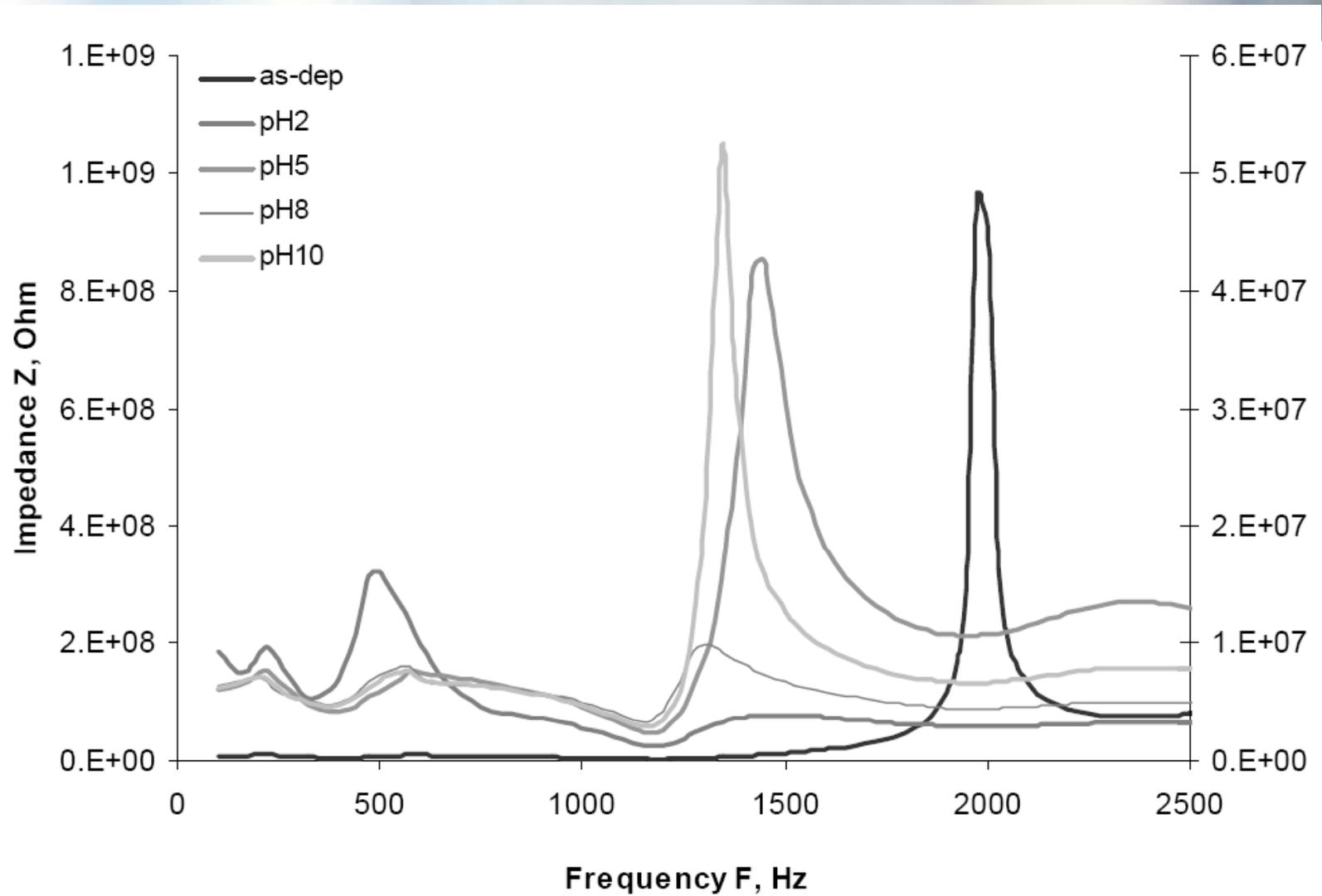
**Change in the resonant frequency and impedance values of the  $Nb_2O_5$  thick film pH sensor.**
